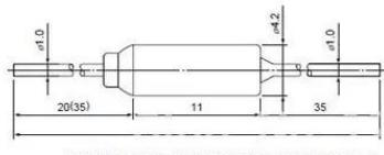
Note: The dimensions for long lead devices are in parentheses.
