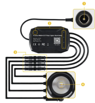
Legende 1. DC 12V input 2. Indicator lights 3. PG - type Connector 4. Inner diameter \varnothing 22mm (PG25) Each Port Max Fiber Optic Cable: 0.75mm—620pcs or 1mm—300pcs
