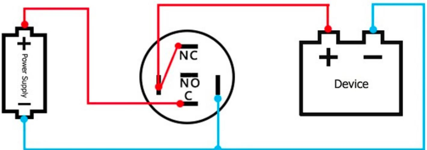
**RÉTROÉCLAIRAGE PERMANENT, INACTIF QUAND APPUYÉ, Contact - NC**
