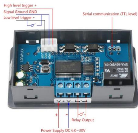
DC 6.0~30V Wiring Diagram
