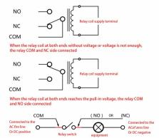
When the relay switch is closed, the device has a voltage at both ends, can work properly, switch off does not work
